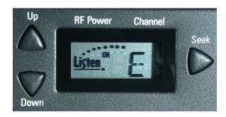
Channel: This indicates the currently tuned channel. See "Which channel should I use?" below for more information and the Channel Selection Chart on page 22.
