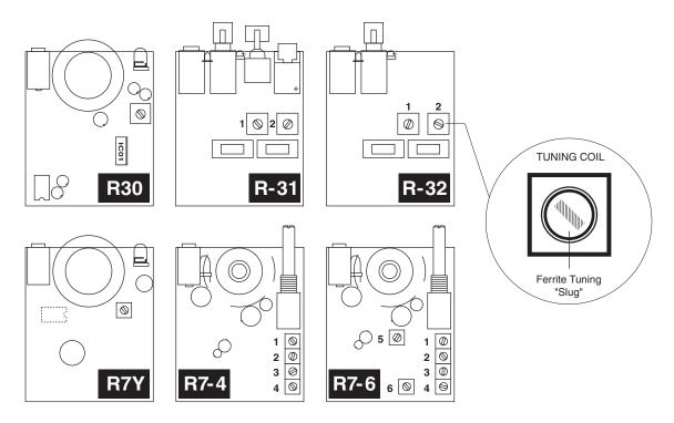
Most Williams Sound single channel Receivers are set at the factory to 72.9 MHz. The standard four-channel receivers (R7-4NA), Channels 1-4, are usually set to frequencies 72.1, 72.5, 72.9, 75.7 MHz respectively. The standard six-channel receivers (R7-6N), channels 1-6, are set to frequencies 72.1, 72.5, 72.9, 75.7, 74.7 and 75.3 MHz respectively.
