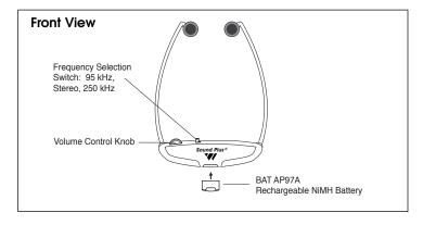
A dual detector infrared "eye" is located in the front of the receiver. Do not cover it up or you will lose reception. Make sure the "SOUND PLUS" label is facing away from you when you put the receiver on.
